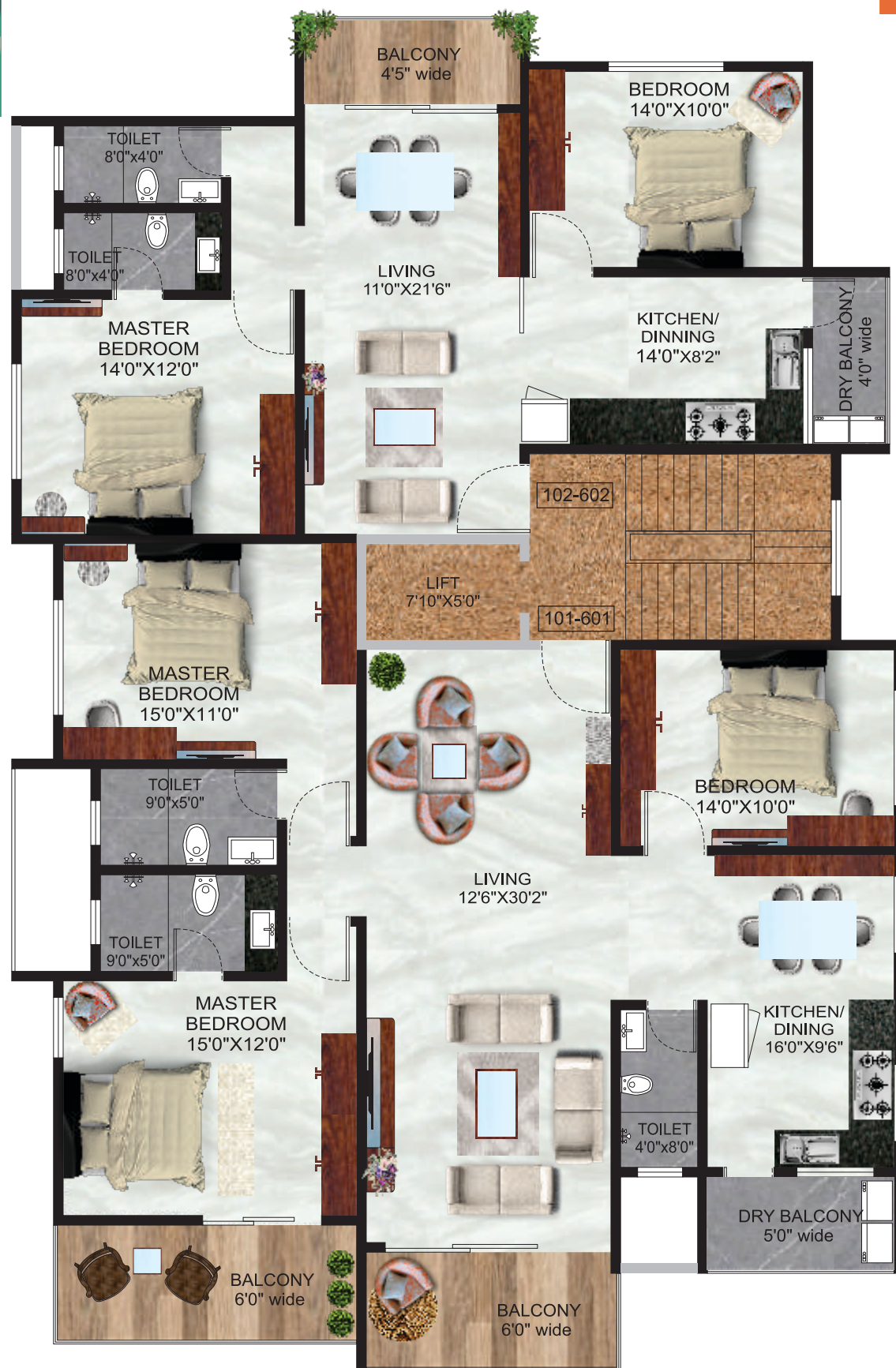
TYPICAL FLOOR PLAN – 1 ST TO 6 TH FLOOR
